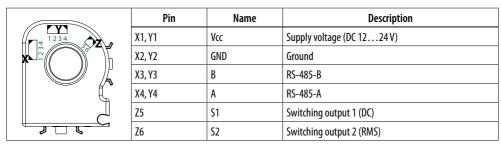
The two four-pole connectors **X** and **Y** are designed as combinations of socket and plug, the two-pole connector **Z** is designed as push-in terminal.
