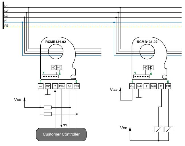
The maximum cable length must be limited to  $\leq$  10 m.
